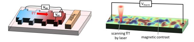
Figure 1- Experimental setup for magneto-thermal transport measuremenst. (a) Thermal gradient applied globally in the sample plane. (b) Thermal gradient applied locally by laser beam enabling a spatially resolved magnetic characterization.
